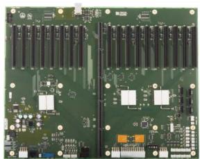
Design of the BERTA 18X computer has been optimized for large number of PCIe type high speed (x16) expansion slots. It offers excellent air flow cooling of option cards and it is highly reliable to minimize down time. Longevity of supply is assured by Intel SKYLARK Xeon processors. Supply of this computer is expected until 2024.
