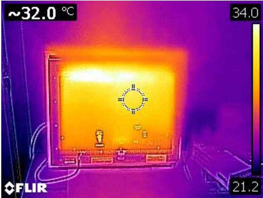
Thermal image of the TR-5197 half fanless computer demonstrates convection air flow with heat rising to the top.
